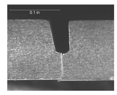
Figure 3 shows the precrack slot and fatigue crack after initial growth. Side view at 2.5X
