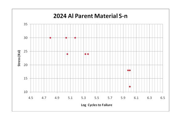
Figure 5 shows current results: The S/N data for the parent material. This will be used as a comparison.
